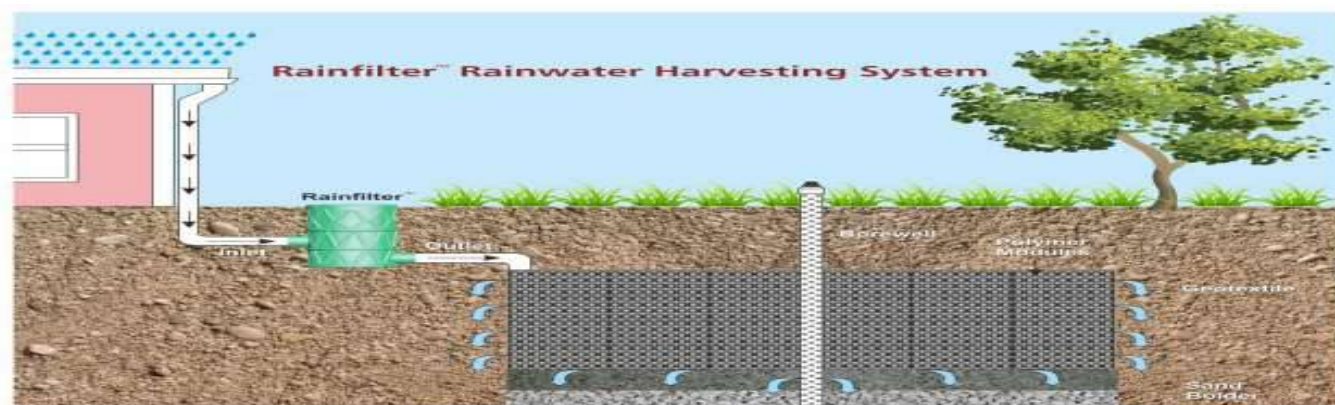
A SCHEMATIC DIAGRAM OF A RAINWATER HARVESTING UNDERGROUND TANK
